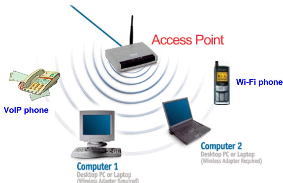
IEEE 802.11 network infrastructure with Wi-Fi devices connected wirelessly via Access Point (AP) or wireless router for data transmission
